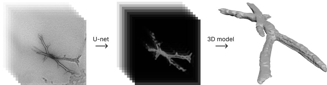
Figure 3.8: To utilise U-net to create a 3D model, it is necessary to split each organoid into single 2D files, crop and ideally drift-correct. These single slices can then be fed to the python script (see the entire code in detail in the appendix B).
